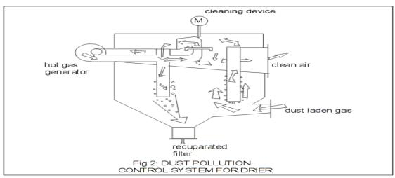
In figure 2 the drier is provided with a bag house filtration system. It features the principle of Reverse Air Cleaning.
